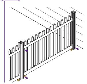
▶ Repeat in the remaining corners using (3) total 3½" self-drilling stainless steel screws.
